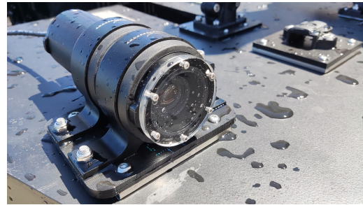
(b) Droplets of water on the camera cage after. This is another barrier to the usage of visual sensors on ASVs.
