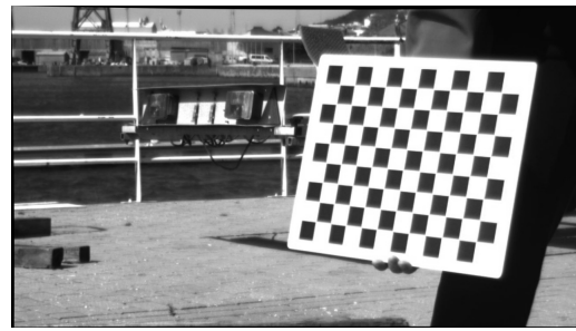
(b) Image frame 3.5a after calibration. Notice the appearance of dark borders.
