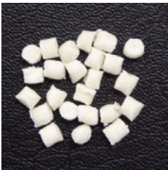
High-density cellulose fiber molding material
