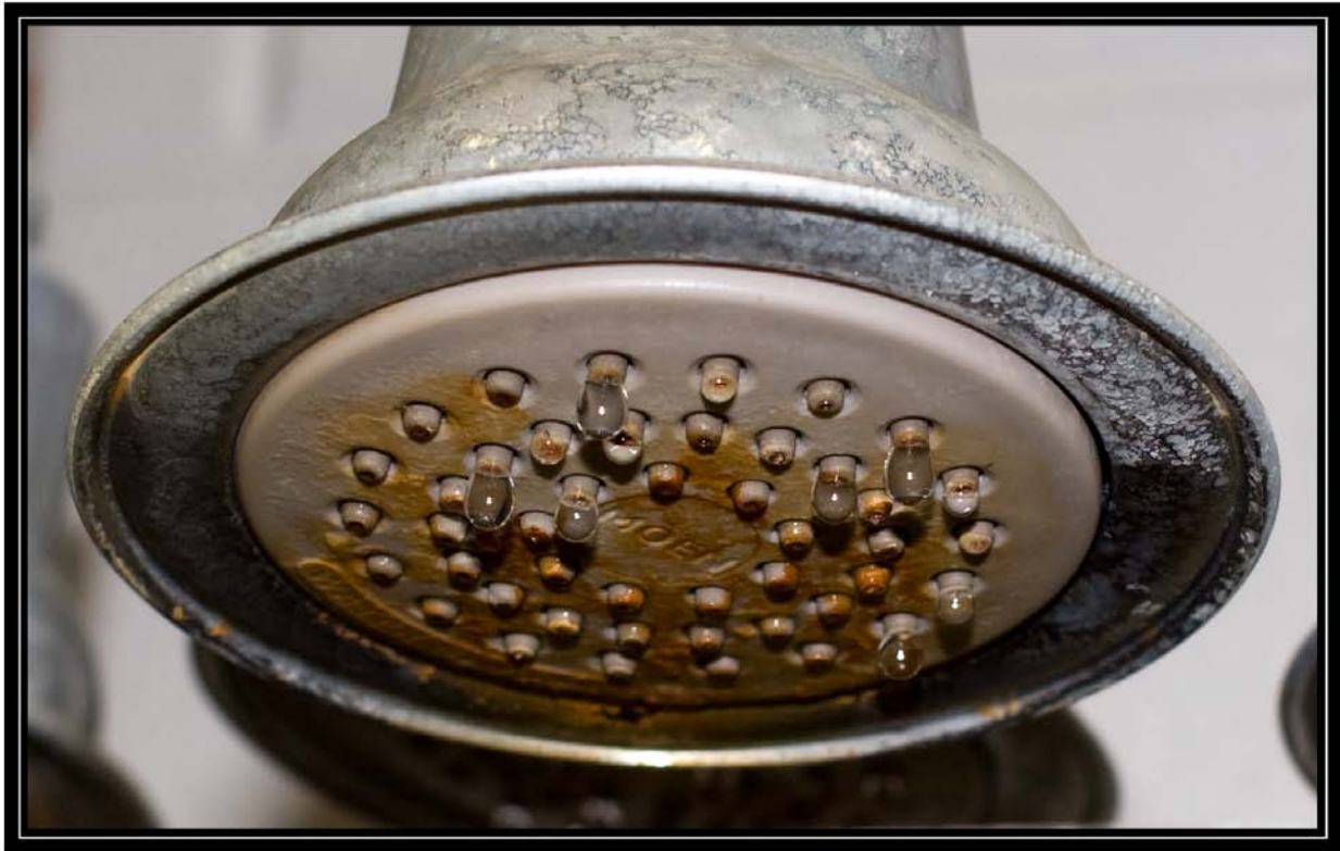
Figure 6-7C. Showerhead 7 on seventh day of testing with hard well water (28 grains per gallon) showing condition of nozzles. Battelle testing for Water Quality Association. May 1, 2009
