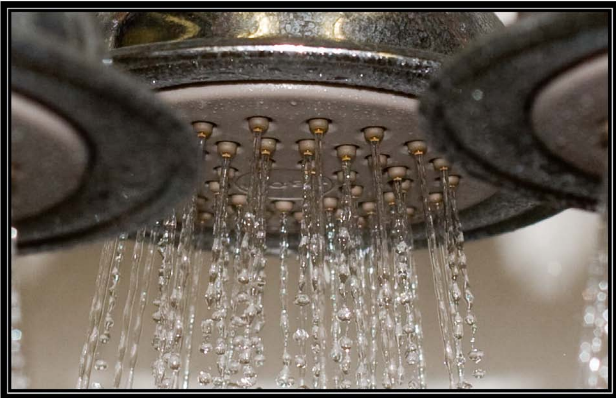
Figure 6-4D. Showerhead 4 on seventh day of testing with soft well water (<1 grain per gallon) showing spray pattern. Battelle testing for Water Quality Association. May 1, 2009
