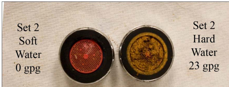
Figure 5-20. Photo showing the Set 2 faucet strainers at the end of the test.
