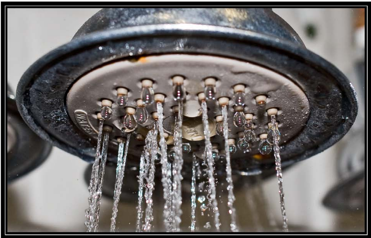
Figure 6-6B. Showerhead 6 on fourth day of testing with hard well water (25 grains per gallon) showing spray pattern. Battelle testing for Water Quality Association. April 28, 2009
