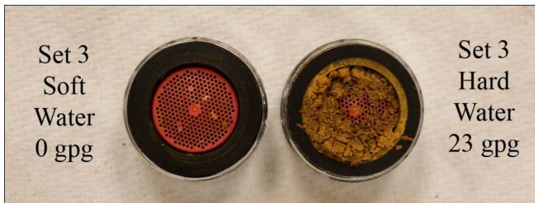
Figure 5-21. Photo showing the Set 3 faucet strainers at the end of the test.
