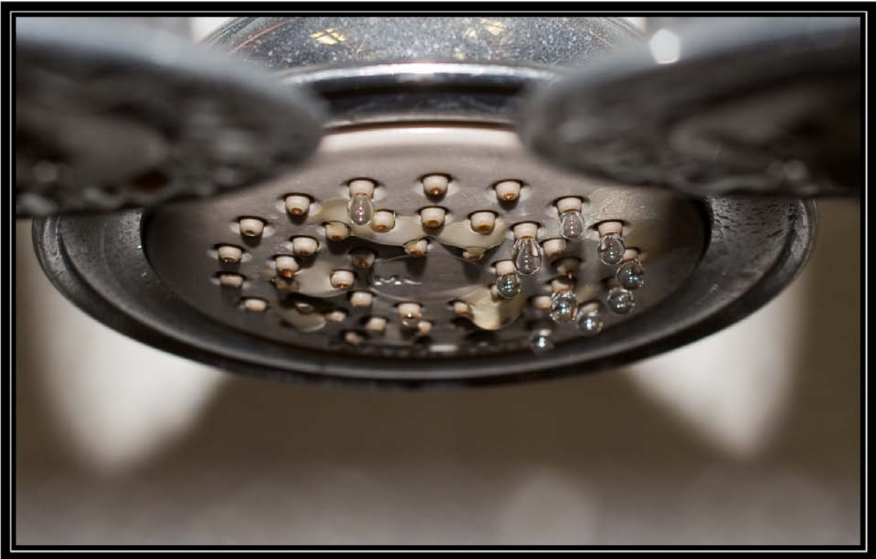
Figure 6-9A. Showerhead 9 on fourth day of testing with hard well water (25 grains per gallon) showing condition of nozzles. Battelle testing for Water Quality Association. April 28, 2009
