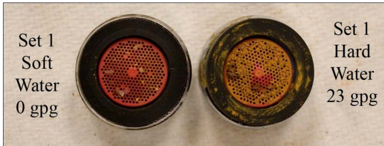
Figure 5-19. Photo showing the Set 1 faucet strainers at the end of the test.
