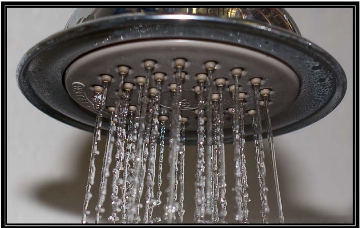
Figure 6-3B. Showerhead 3 on fourth day of testing with softened well water (<1 grains per gallon) showing spray pattern. Battelle testing for Water Quality Association. April 28, 2009
