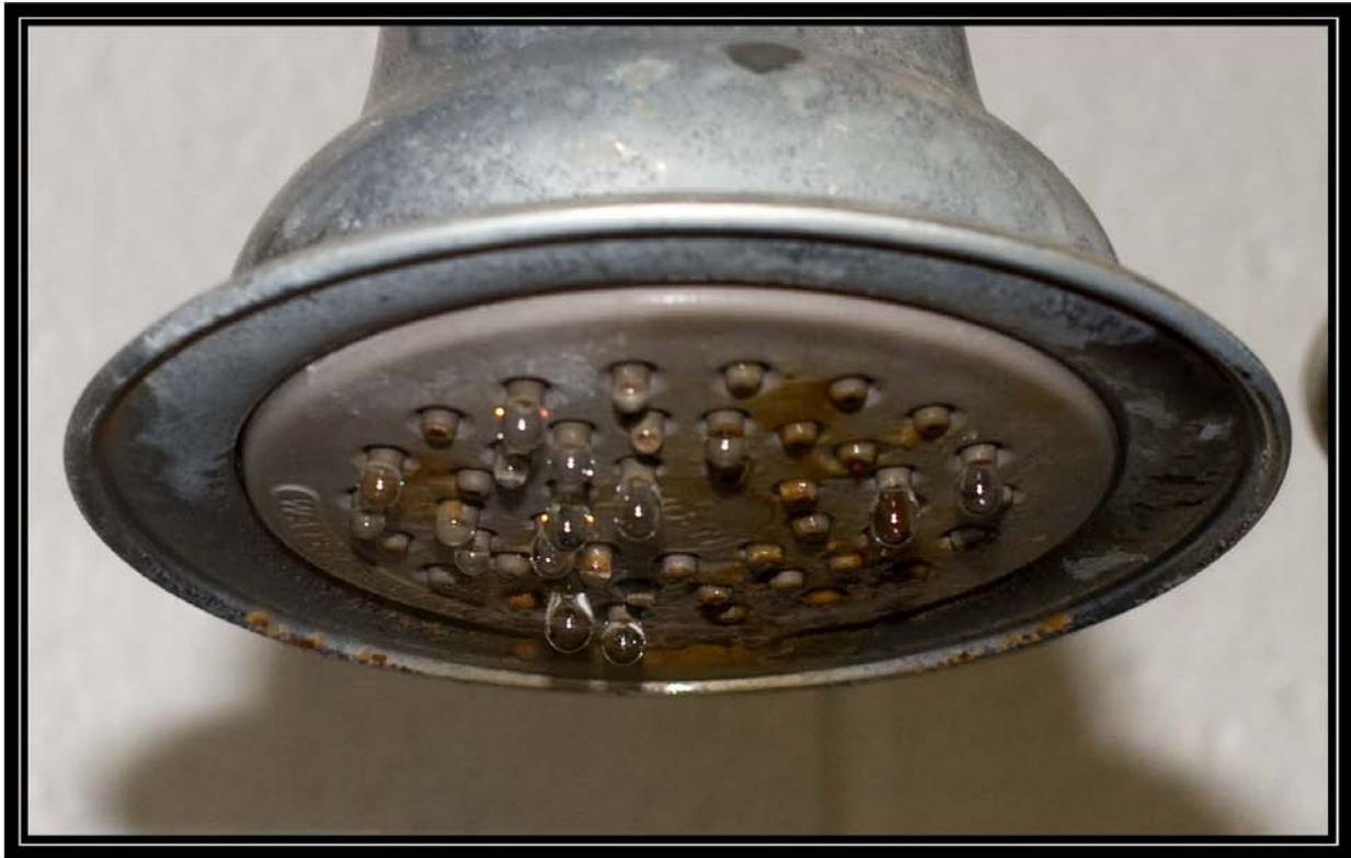
Figure 6-8C. Showerhead 8 on seventh day of testing with hard well water (28 grains per gallon) showing condition of nozzles. Battelle testing for Water Quality Association. May 1, 2009
