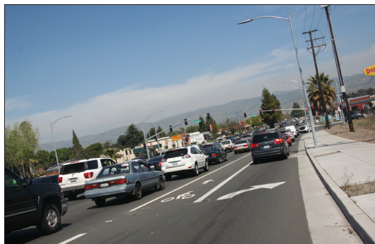
This bike lane on Tully Road enables bikes to pass the queue of right-turning cars in the right-turn only lane.
