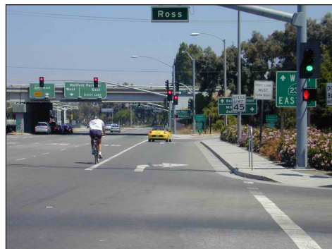
This bicyclist approaching an interchange has to squeeze between the through lane and the right-turn lane since there is no bike lane.
