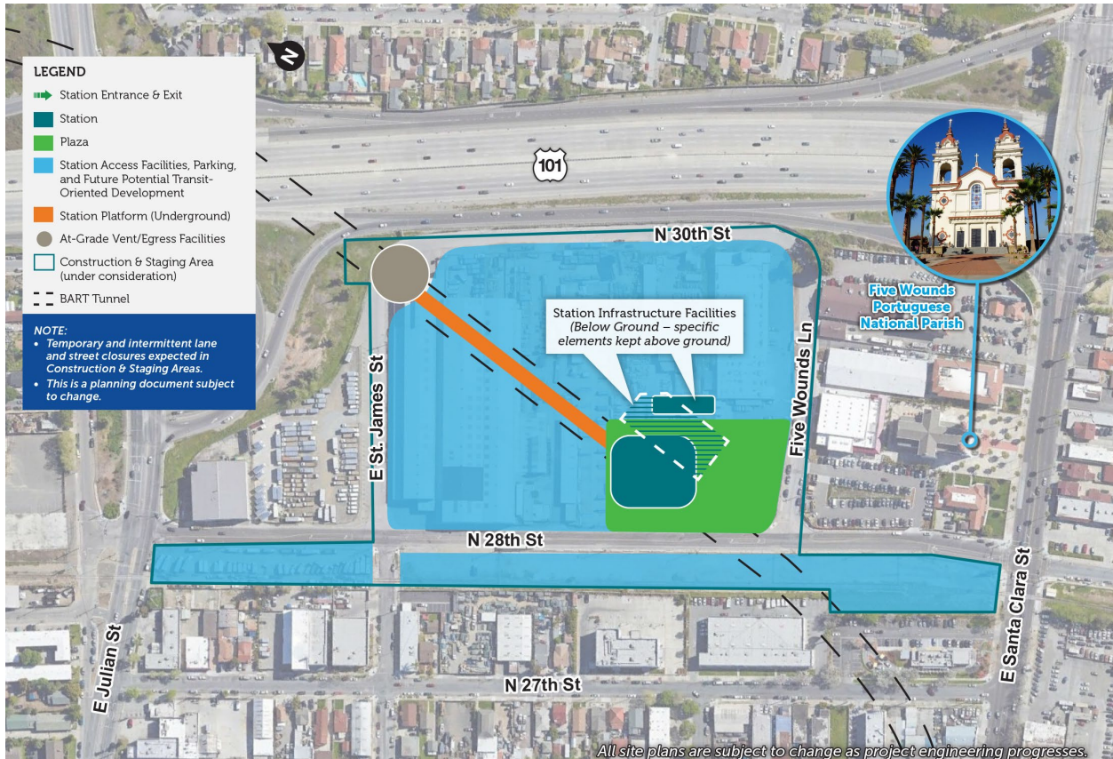
Figure 6: 28th Street/Little Portugal BART Station – Draft Sketch of Station Infrastructure Facilities Primary Option (Below Ground)
