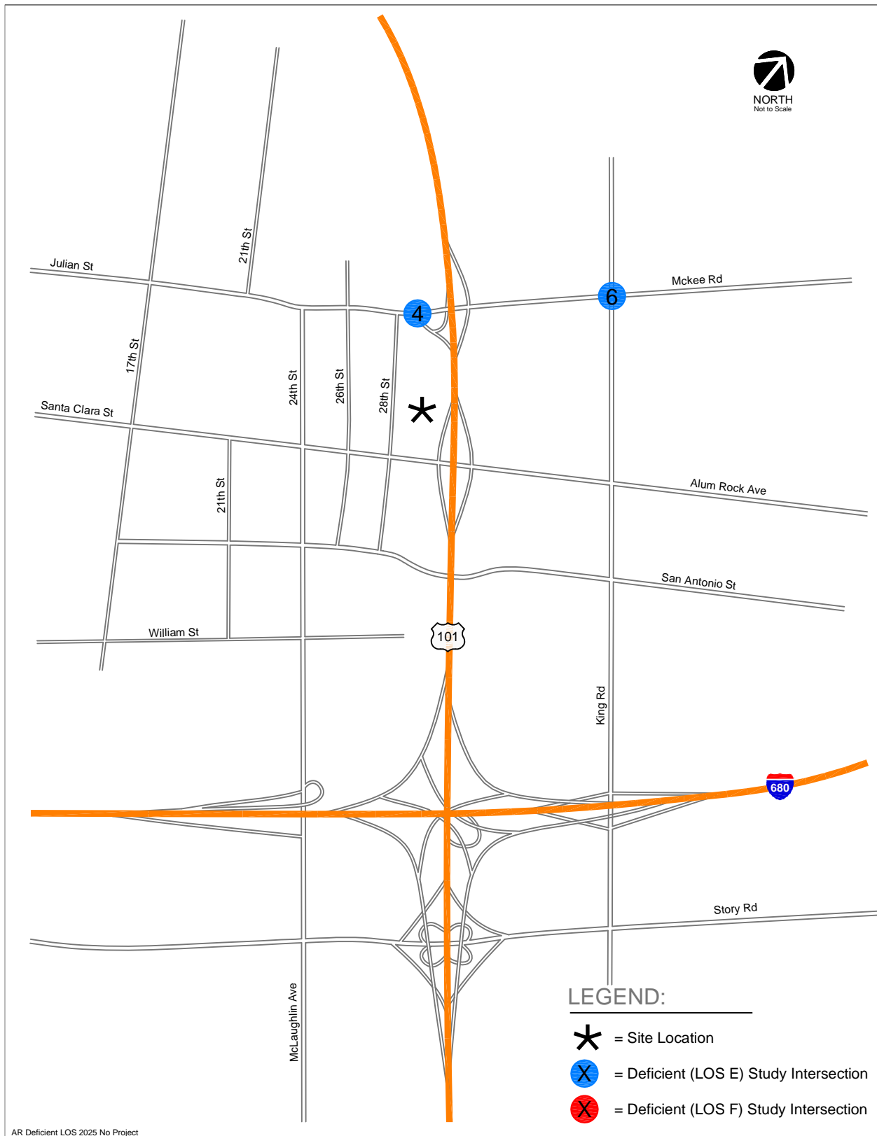
Figure 26 2025 No Project/Phase I Conditions Deficient LOS Intersections – Alum Rock/28 th Street Station
