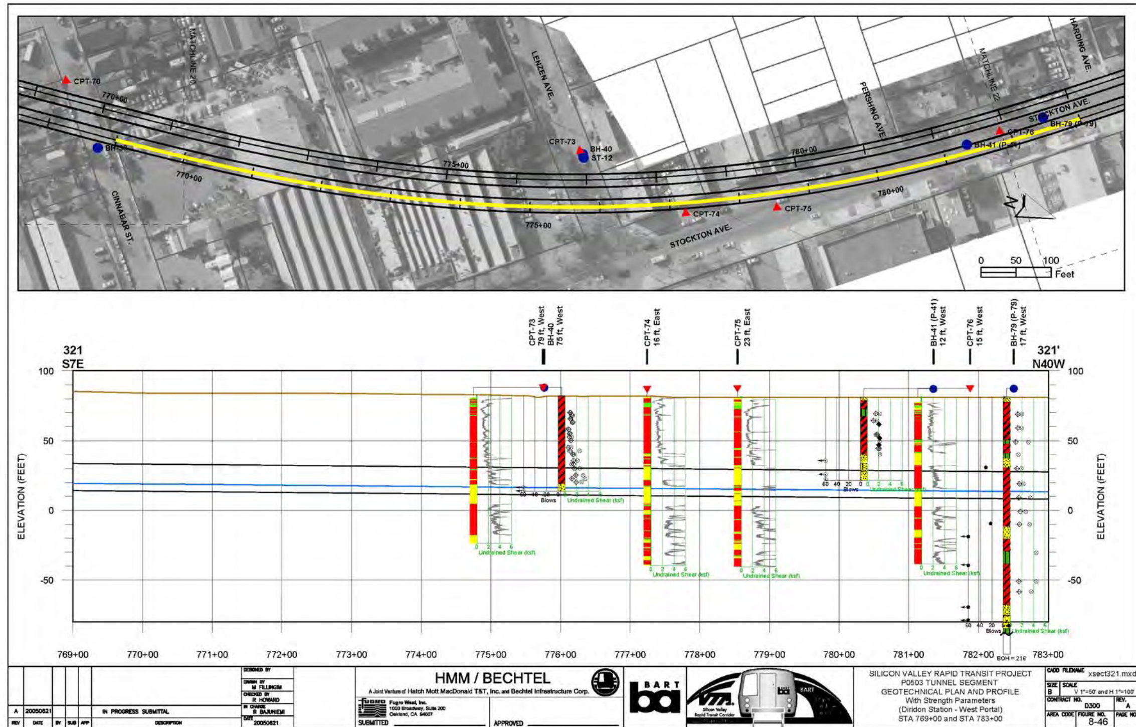
Figure 8-46. Geotechnical Plan and Profile with Strength Parameters: 769+00 to 783+00.
