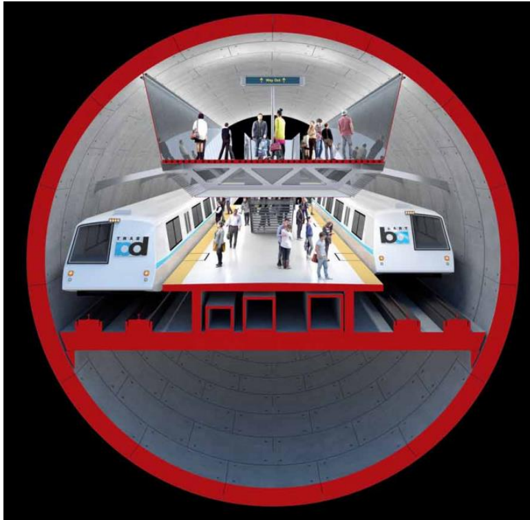
Concourse & Platform in Tunnel
