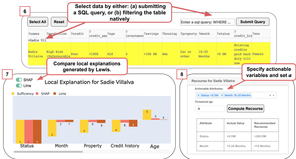
Figure 3: A snapshot of local explanations generated by LEWIS. (6) The user can select a sub-population (context) or a particular data point specified in the form of a SQL query as SELECT * FROM data WHERE context or filter the table in place; (7) shows the contextual or local explanations generated by LEWIS for the use case selected in (6) along with feature rankings; (8) If the individual selected in (6) received a negative decision by the black-box algorithm, then LEWIS allows the user to specify the set of actionable variables and a threshold for sufficiency, and generates appropriate recourse.
