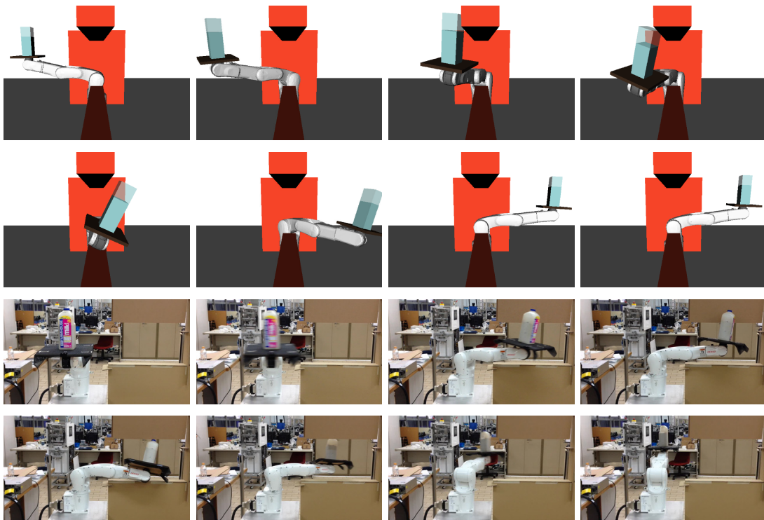
Figure 9: Snapshots of the motion of Fig. 8B–E taken every 0.5s. Top two rows: front view of the motion in the simulation environment. Bottom two rows: side view of the motion executed on the actual robot (see also the video at http://youtu.be/LdZSjNwpJs0 ).
