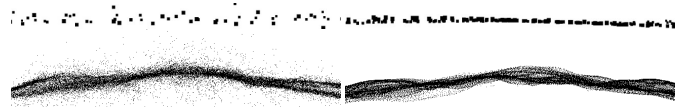
Fig. 12. Cut through surfaces from ElasticFusion (top left) and [36] (bottom left) compared to corresponding surfels in our approach (right). Our method generates smoother surfaces due to our denoising steps (Sec. 3.2).
