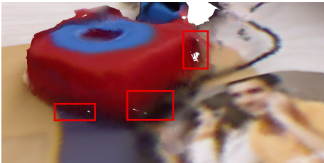
Fig. 18. Example of tiny holes (highlighted in red) in a close-up of the reconstruction of fr1/desk [44] which is also shown in Fig. 13. The holes are created since the reconstructed surfels are too noisy for meshing in these areas. While they are usually tiny, they can be quite noticeable if the mesh is rendered without anti-aliasing.
