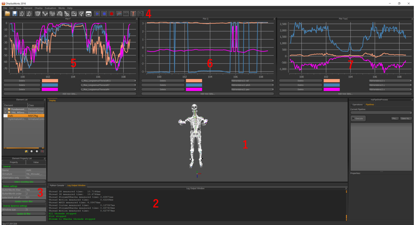
Fig. 8. DhaibaWorks with the integrated plugin. The plugin adds several tools to the main window. It adds 1) visualization of the musculoskeletal model, 2) information into the console on the state of the software, 3) tunable parameters such as filters, 4) toolbar buttons to easily play, record, initialize the software 5-7) plots to visualize on-line state. 5) show 3 back muscles (Longissmus Thoracis 11, 7, 4), 6) is the rib vertebra 12 orientation (roll, pitch, yaw) and 7) show joint reaction forces of the rib vertebra 12 (x, y, z).
