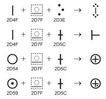
If a rendering system cannot display obligatory bi-consonants with the correct, fully-formed bi-consonant glyphs, a fallback rendering should be used which displays the TIFI-NAGH CONSONANT JOINER visibly, so that the correct textual distinctions are maintained, even if they cannot be properly displayed.
