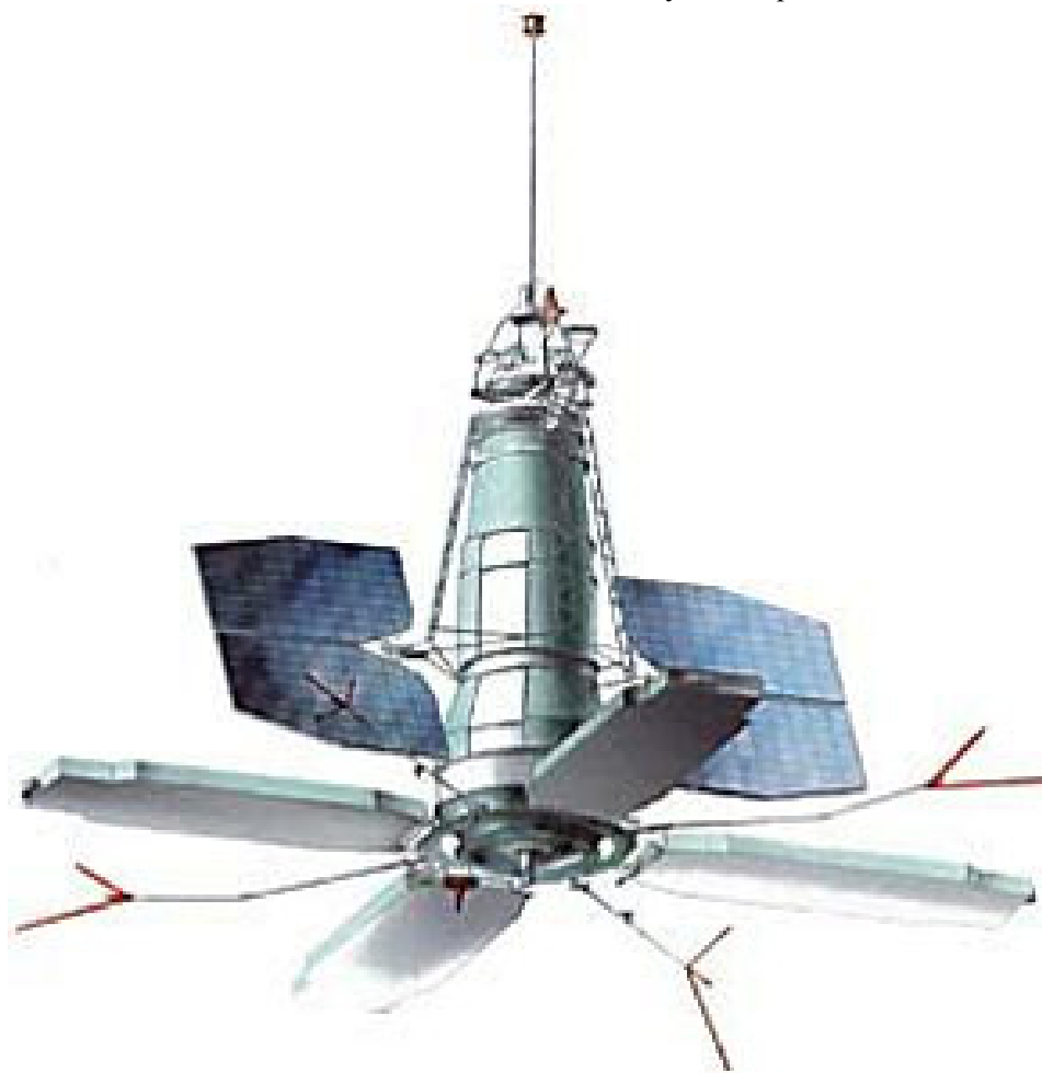
Figure 18: Image of similar Tselina-R satellite (credit: Yuzhnoe). This gives a clearer view of the elint antenna 'paddles'. However, the four forked boom antennae may be unique to the Tselina-R model.
