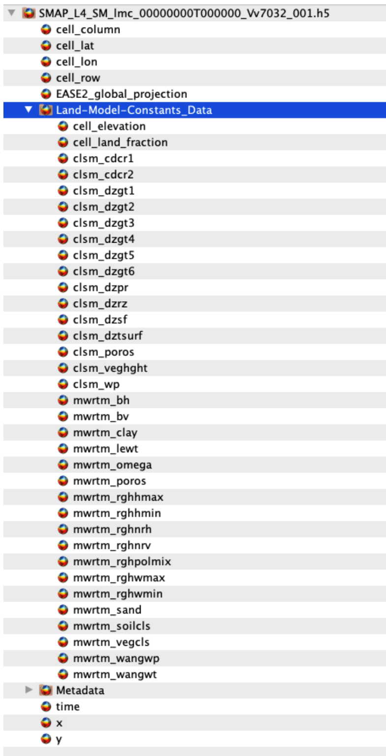
Figure 3. Contents of a Land Model Constants file. For a complete list of file contents for the SMAP Level-4 soil moisture product refer to the L4_SM Product Specification Document (Reichle et al., 2022a) available in the Documentation section of the landing page. Data Fields
