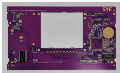
▲ Straight from Mathijs Nilwik's garage in the Netherlands: a Game Gear main board. Perfect for bringing a dead system back to life.
