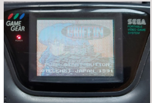
▲ With the capacitors replaced, the sound works and the image is much brighter. I still need to replace this broken old screen, though.
