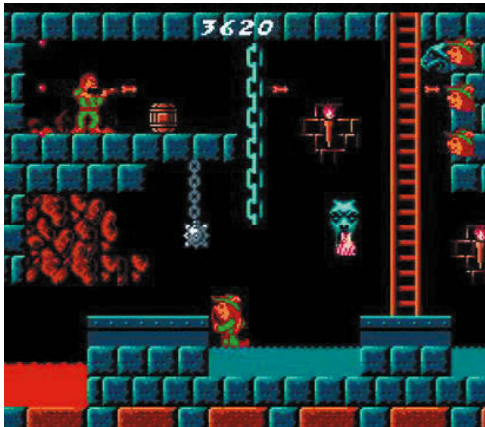
^ The score was placed high on the screen so as to avoid a clash with other sprites on the same horizontal line.
