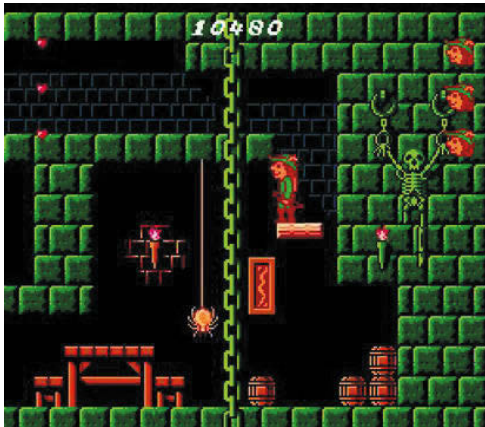
^ Super Robin Hood saved memory by reusing some background sprites with different colour palettes, like the stone blocks you can see here.
