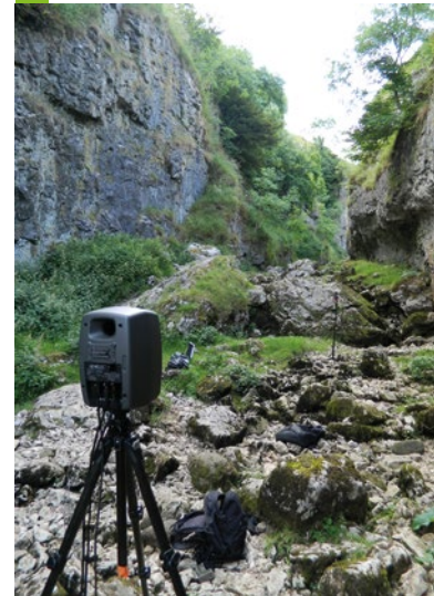
^ Capturing the reverberant 'impulse response' of the narrow rock-pass at Troller's Gill in three dimensions, for the openairlib.net research project. Spot the mic and laptop?
