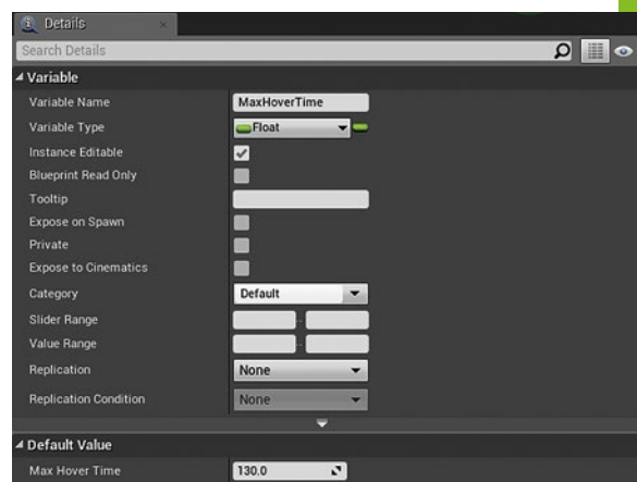
The details panel for the variables will let us set not only the type and default values for variables, but what category they will appear in, or if the value has min and max limits.
