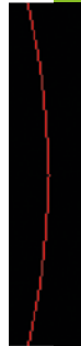
> Figure 5: See that pixel in the middle of the curve? We can avoid this - and draw a smoother curve - by clipping our maximum and minimum SIN values.
