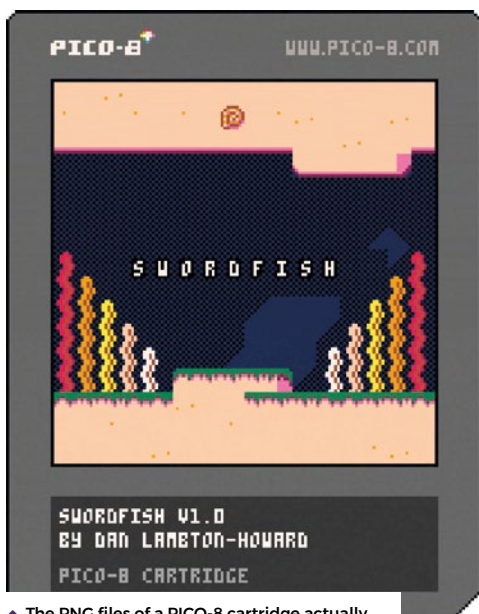
▲ The PNG files of a PICO-8 cartridge actually contain the entire game encoded within them. And they're cute, to boot.
