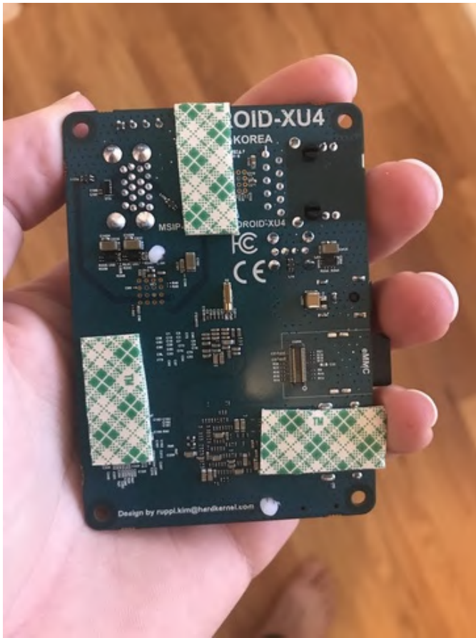
Figure 9 - Double sided mounting underneath the ODROID-XU4
