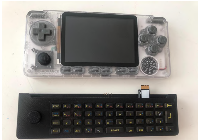
Figure 10 - Keyboard not attached, showing the microSD extension
