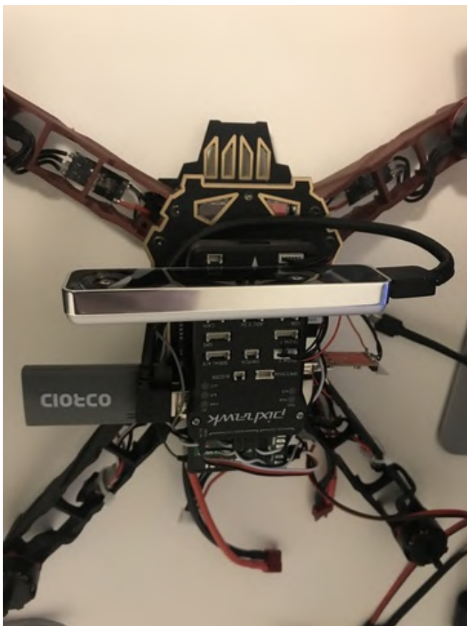
Figure 13 - Realsense T265 camera mounted on top of the Pixhawk FCU and connected to ODROID
