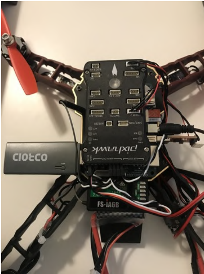
Figure 12 - Receiver, barrel jack, USB-TTL, WiFi adapter, and ESC outputs connected
