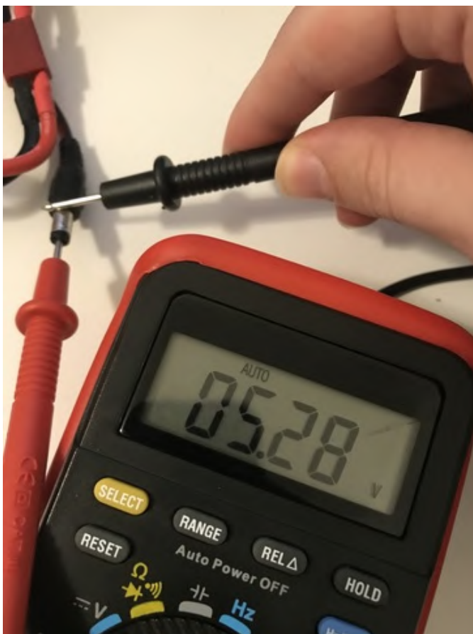
Figure 7 - Voltage output from the BEC after powering on the circuit
