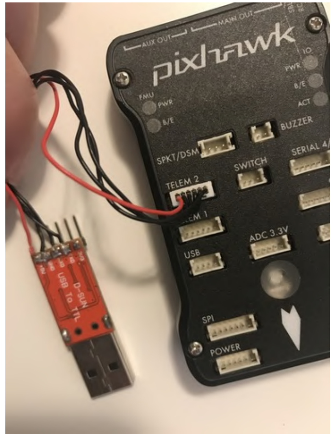
Figure 8 - USB-TTL data connection to Pixhawk
