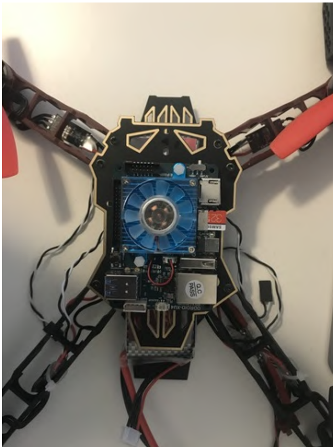
Figure 10 - The ODROID mounted on the Q330 frame
