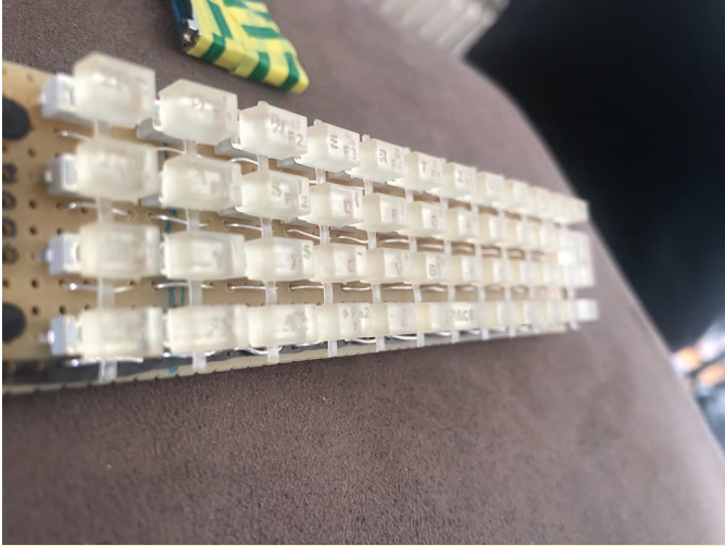
Figure 5 - The printed keys, before the next step of painting them black
