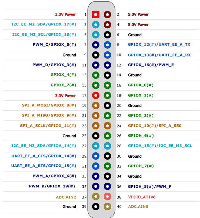
Figure 16 - GPIO Header
