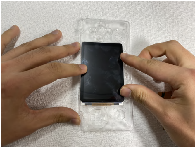
Figure 20 - Closeup of removing the double-sided tape
