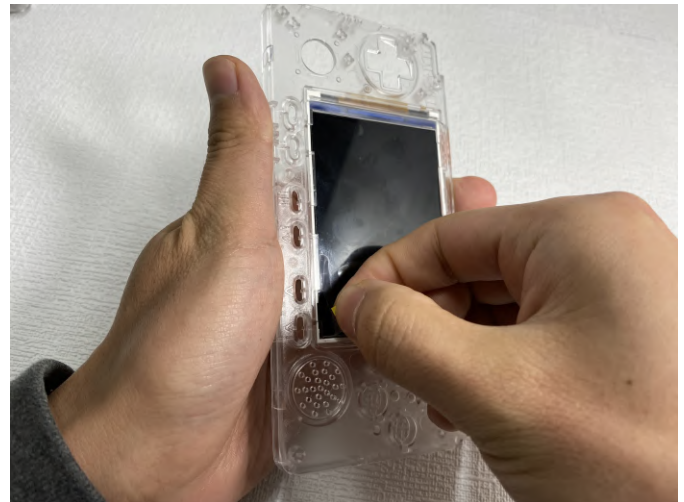
Figure 17 - Closeup of removing the double-sided tape
