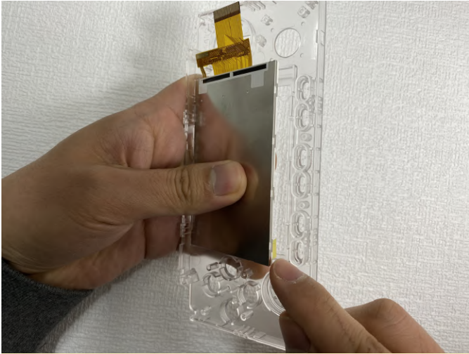
Figure 8 - Closeup of LCD panel insertion
