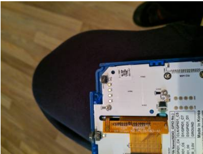
Figure 4 - Another view of the board with SW15 accidentally removed
