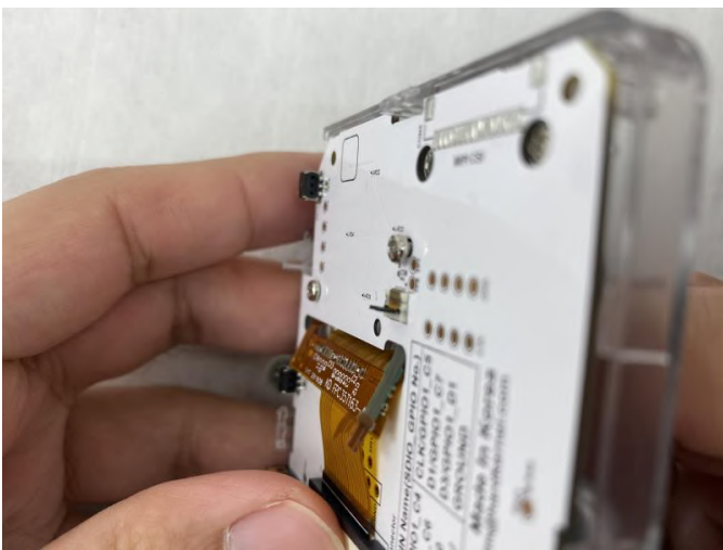
Figure 46 - Closeup of attaching the PCB connections
