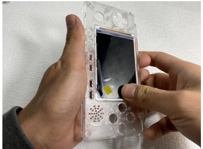
Figure 12 - Make sure that the yellow tab is in front of the enclosure
