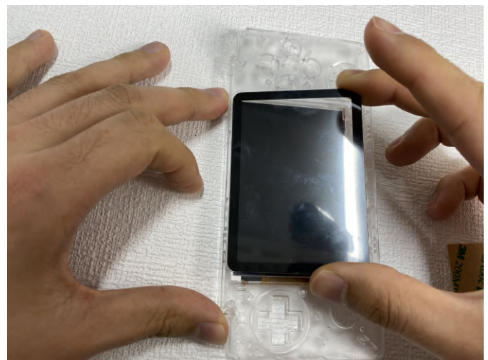
Figure 19 - Closeup of removing the double-sided tape
