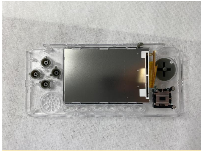
Figure 29 - Closeup of attaching the buttons
