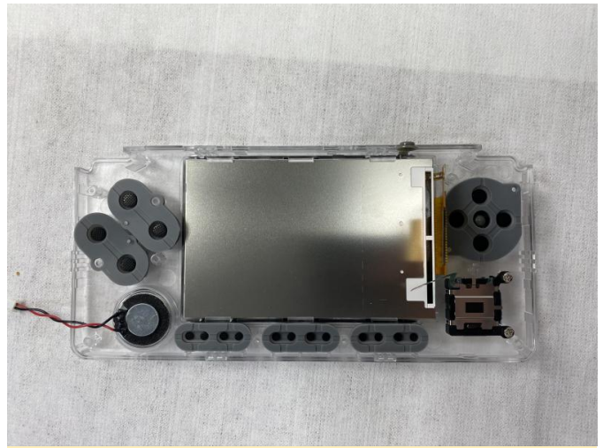
Figure 35 - Closeup of speaker assembly
