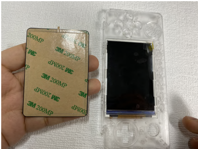
Figure 15 - Closeup of removing the double-sided tape
