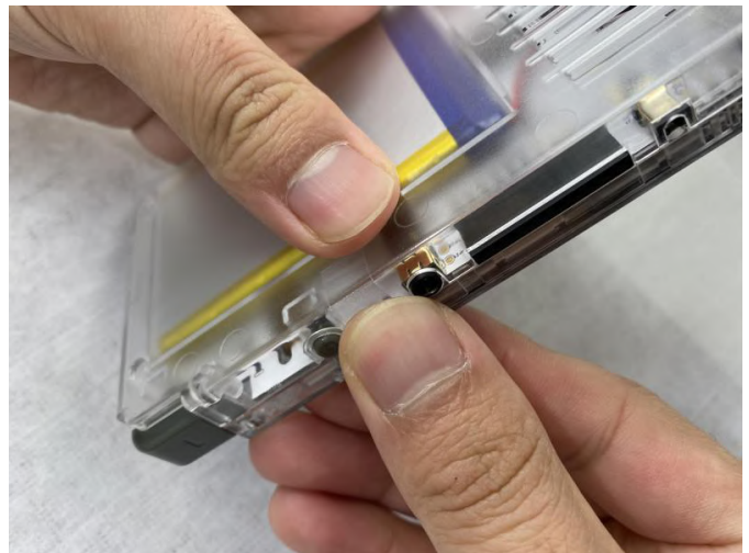
Figure 66 - Closeup of attaching the enclosure
