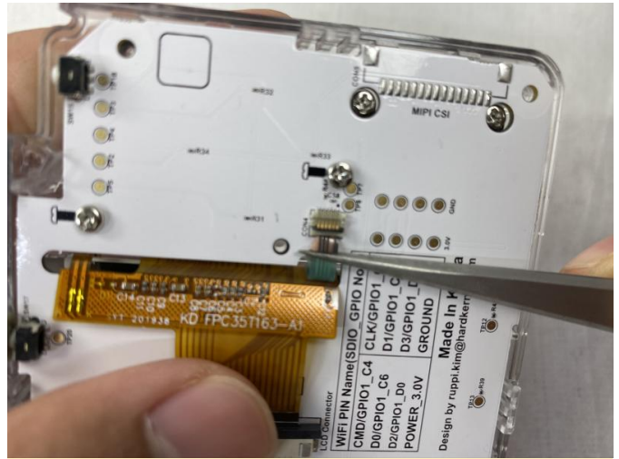
Figure 48 - Closeup of attaching the PCB connections
