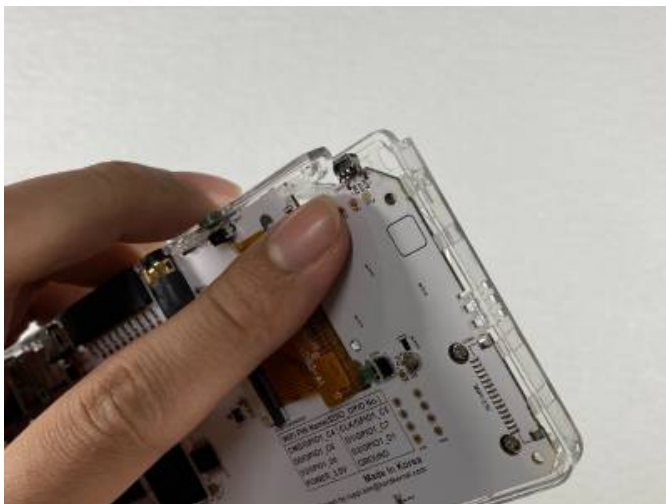
Figure 1 - SW15 can easily be bent during disassembly if care is not taken
