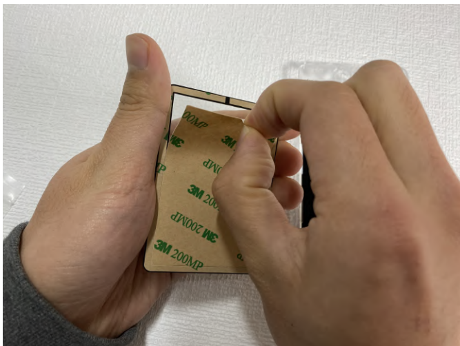
Figure 16 - Closeup of removing the double-sided tape
