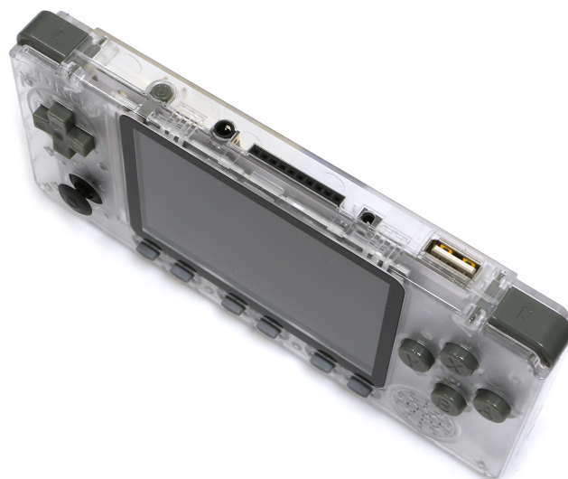
Figure 2 - Lots of ports to call, port-of-call; from left to right: left shoulder trigger, power button, audio output jack, GPIO, power jack, USB 2.0 Host port, and right shoulder trigger. Photograph courtesy of Hardkernel.
