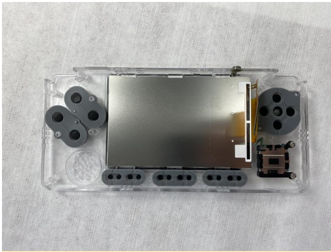
Figure 32 - Closeup of inserting the rubber buttons
