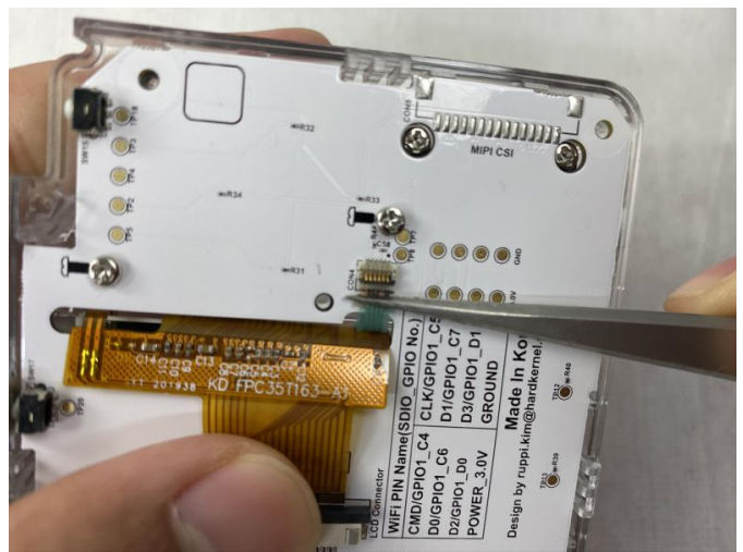
Figure 49 - Closeup of attaching the PCB connections
