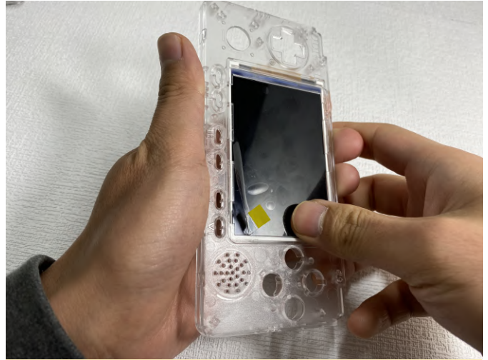
Figure 11 - Closeup of LCD panel insertion
