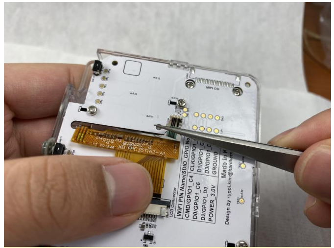
Figure 47 - Closeup of attaching the PCB connections
