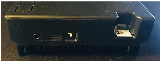
Figure 10 - white switch is set to the right, and SD card is inserted
