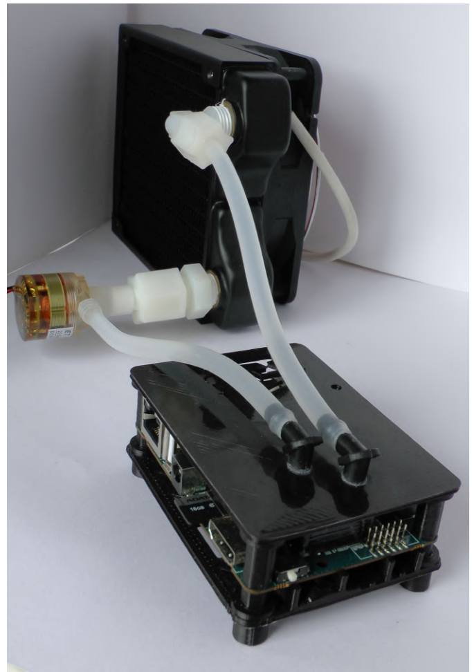
Figure 5 - Waterblock Test Bed
