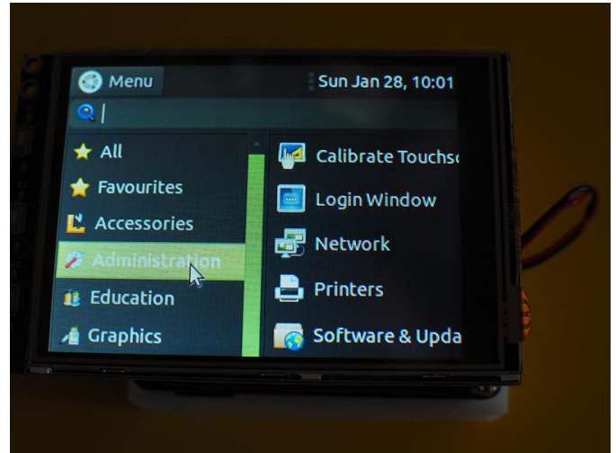
Figure 3 - After you've completed the Hardkernel C1 shield wiki, look for the touchscreen calibration app inside the Ubuntu menu. Run this app for finalizing the touchscreen shield setup.
