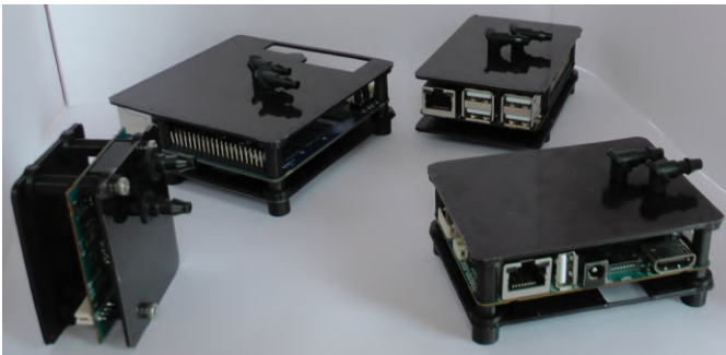
Figure 4 - ODROID Water Cooled Cases (MC1, N1, C2 and XU4)
