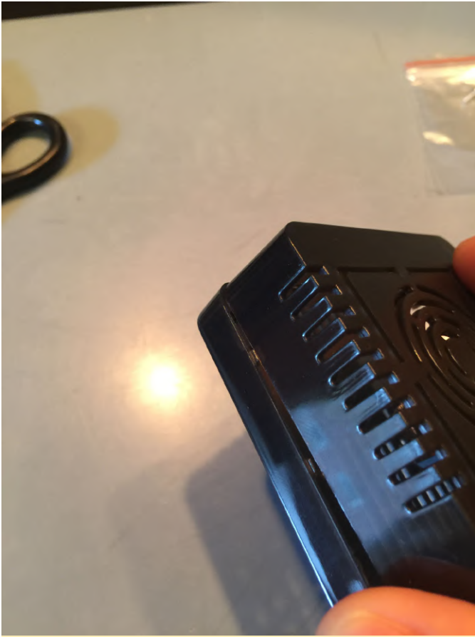
Figure 5 - Case close up of clips along the side
