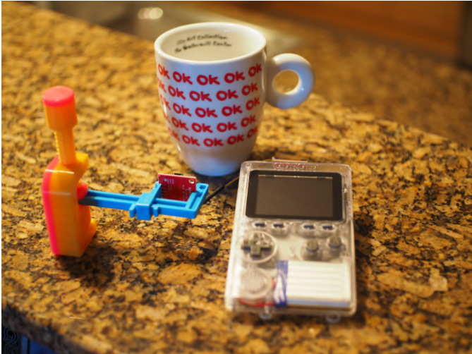
Figure 4 - Here's a handy setup for using your ODROID-GO to measure IR heat
