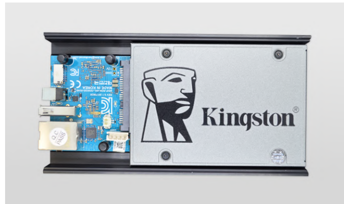
Figure 1 - My ODROID-HC1 BitTorrent Seed Server with a 960GB Kingston SSD
