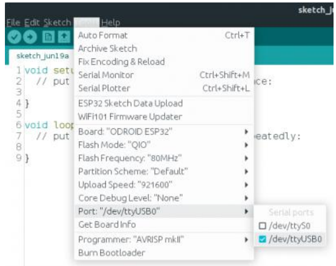
Figure 3 - Selecting a proper serial port in Linux
