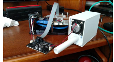
Figure 6 - Inserting the front panel backwards improved the bass response
