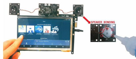
Figure 4 – The Stereo Boom Bonnet speakers can also be separated and attached anywhere with a small amount of glue
