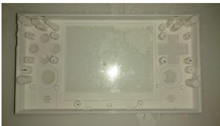
Figures 2 and 3 - Back internal view of the case. You can see batteries space at the bottom and some striations for CPU + GPU thermal dissipation.
