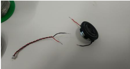
Figure 7 - Don't cut the wires too close to the speakers, in case you have to start over again. Twist the exposed wire-ends together.
