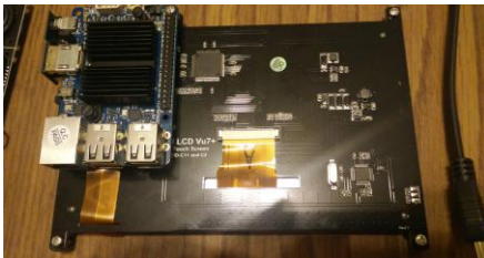
Figure 2 – Attaching the ODROID-C1+ on the back of the Vu7 Plus
