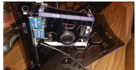
Figure 4 and 5 – I ran out of 20mm spacers and switched to 10mm. It doesn't look pretty. Please use 20mm instead. Don't be as lazy as me.
