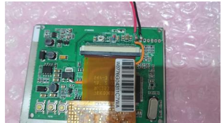
Figure 6 - Closeup of the ODROID 5V wiring
