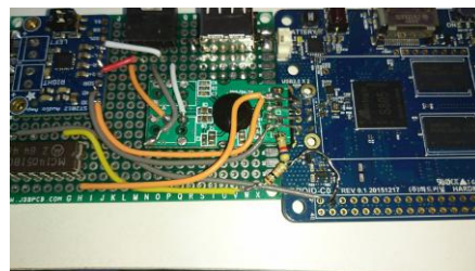
Figures 18 and 19 – Closeup of the analog multiplexer wiring
