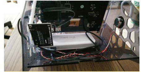
Figure 13 - This 12500 mA battery should give you 3-5 hours of mobile entertainment for gaming, watching movies, or listening to music
