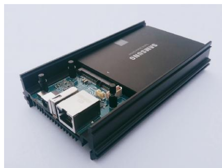
The ODROID-HC1 is an amazing stackable board for building your personal cluster
