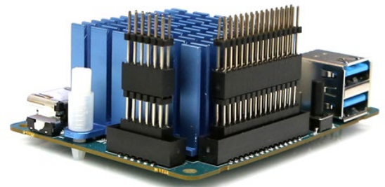
The header extenders can be stacked to make the GPIO pins more accessible
