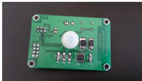
Figure 2a - nRF24 Motion Sensor PCB - Top View
