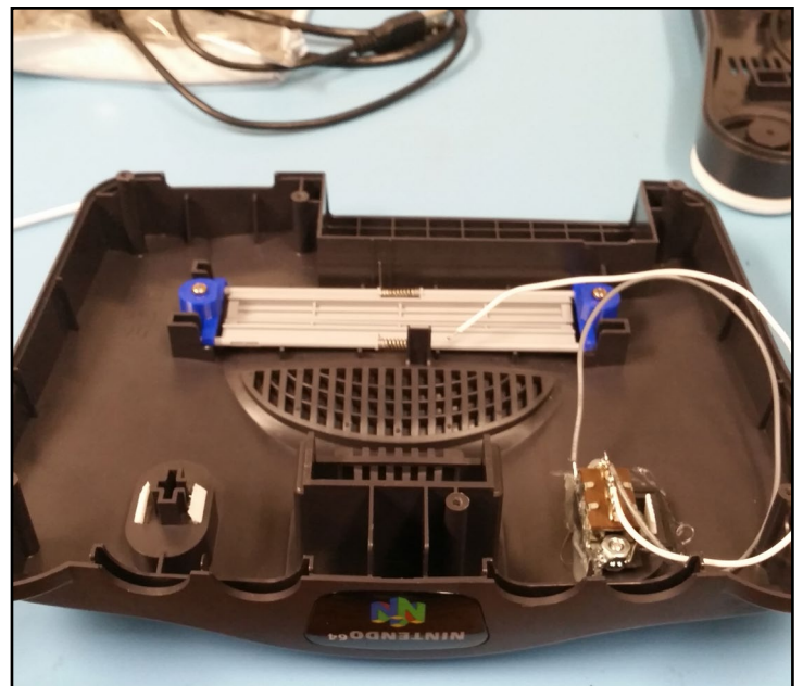
Figure 7 - For the top, I printed the game pack hold downs to make more space inside the console while maintaining the appearance of the Nintendo 64
