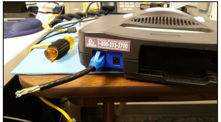
Figure 6 - The rear of the console showing the Ethernet outlet and DC power jack.
