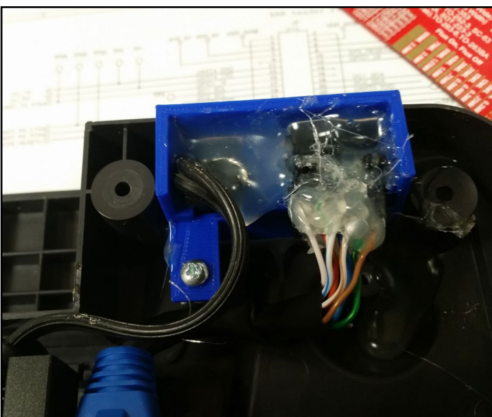
Figure 4 - Ethernet and DC jack are soldered and glued securely, making sure to have the DC jack soldered to the correct polarization before gluing.
