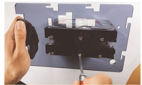
Figure 6 - Screw the left and right pieces to the hard disks (A + B + P)
