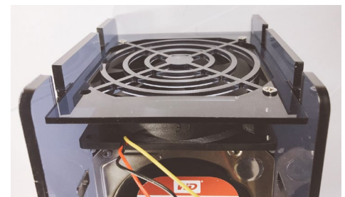
Figure 9 - Assemble the fan and back piece and place the fan at the back side, making sure to use only 3 screws in this step (E + G + N)
