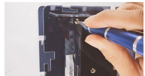
Figure 8 - Screw the CloudShell-2 board to the left and right pieces (O)
