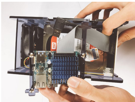
Figure 12 - Connect the GPIO ribbon cable and USB 3.0 cable between the ODROID-XU4 and the CloudShell-2 board (F + H)
