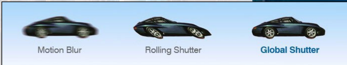
Typical problems in capturing high speed objects. (source: Teledyne DALSA)
