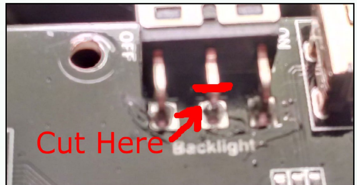
Figure 2 - Middle pin to be cut, of the hardware switch
