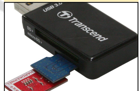
Bottom view of eMMC reader and eMMC module inserted into SD card reader
