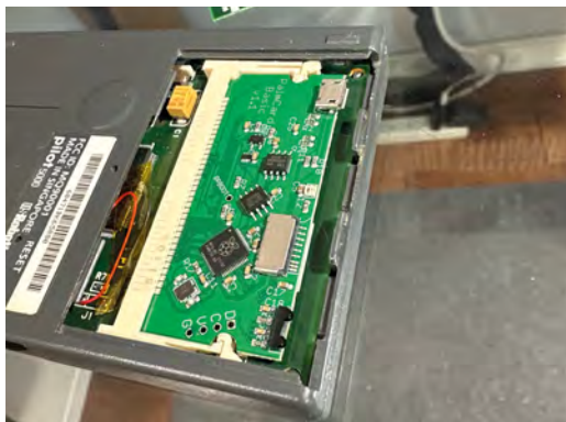
▶ Dmitry has also found a way to wire up external RAM to the RP2040 in a way that it’s writable, readable, and cached ( magpi.cc/romram )
