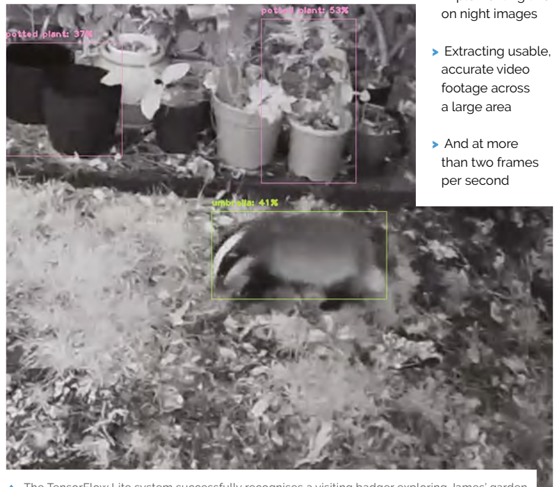
▲ The TensorFlow Lite system successfully recognises a visiting badger exploring James' garden
