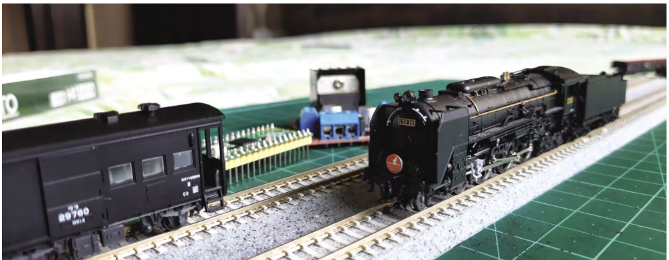
▼ Raspberry Pi Pico reads the track sensor and controls the L298N motor driver connected to the track
