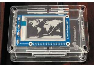
▲ The e-paper display mid-refresh. It takes about three seconds to refresh, but it’s fast enough for this kind of project
