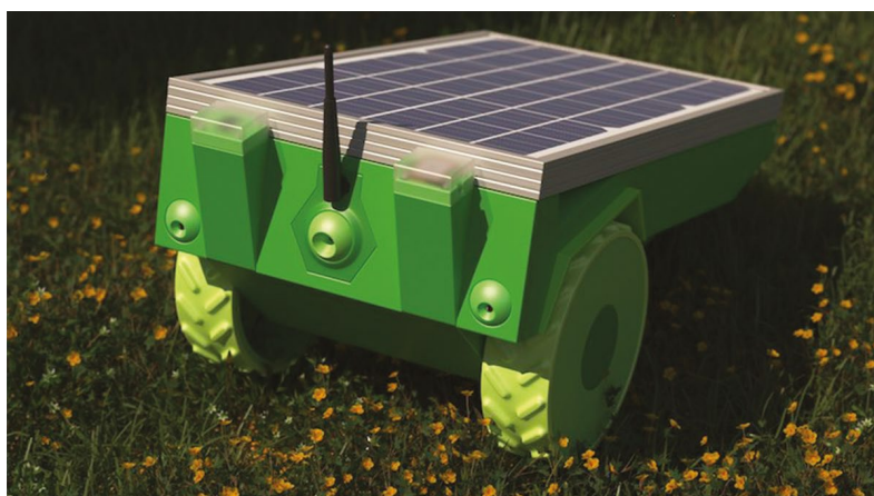
▲ A prototype version of PiMowBot shows off its generous solar panel
