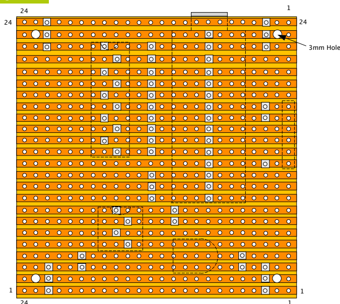
► Figure 5 Back track breaks on the data acquisition module
