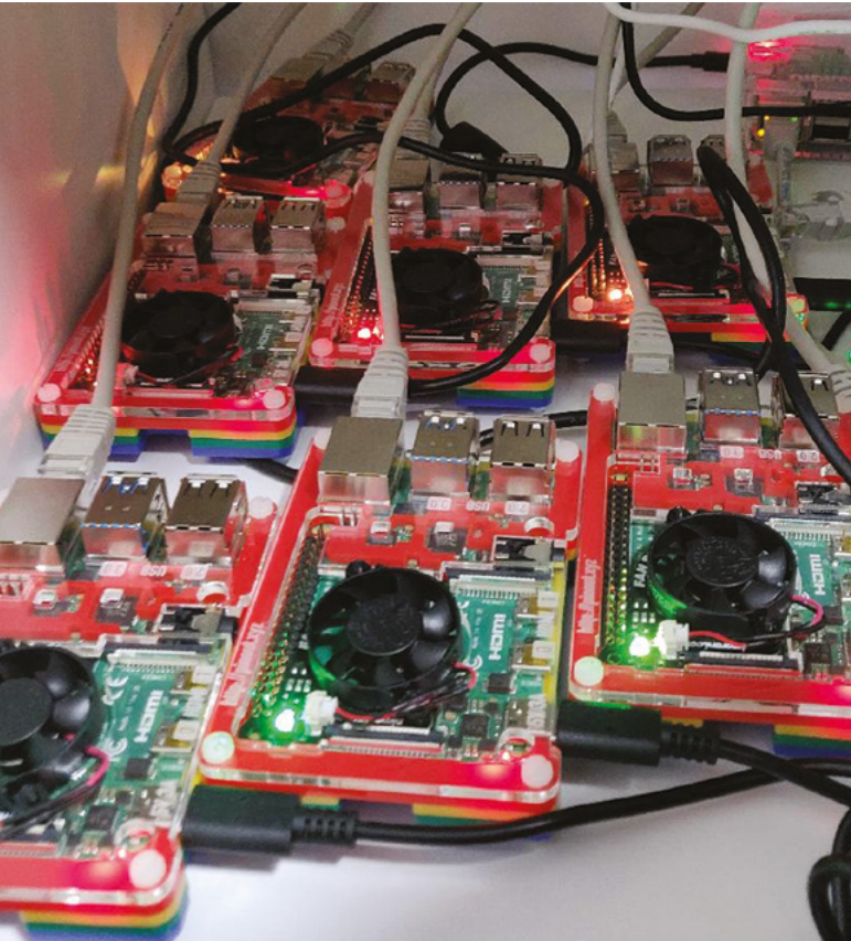
▲ Here is Igalia's Continuous Integration system that's used for running regression tests
