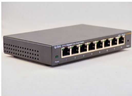
▲ A dedicated inexpensive switch will speed up communications. Raspberry Pi 4 computers can take advantage of full-bandwidth Gigabit Ethernet
