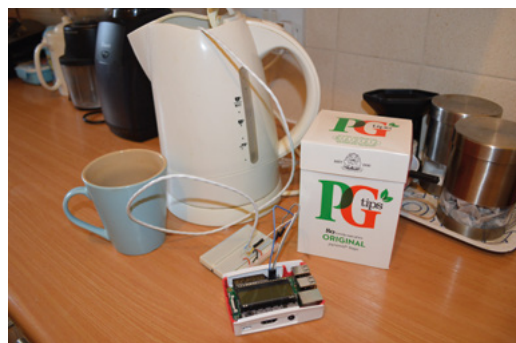
▲ You can take the temperature of water in a kettle and be alerted by a buzzer when it has boiled
