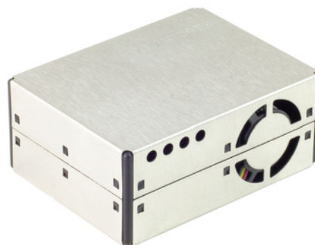
▲ Available separately, the PMS5003 sensor measures the number of tiny particles – up to 1, 2.5, and 10 microns – in the air
