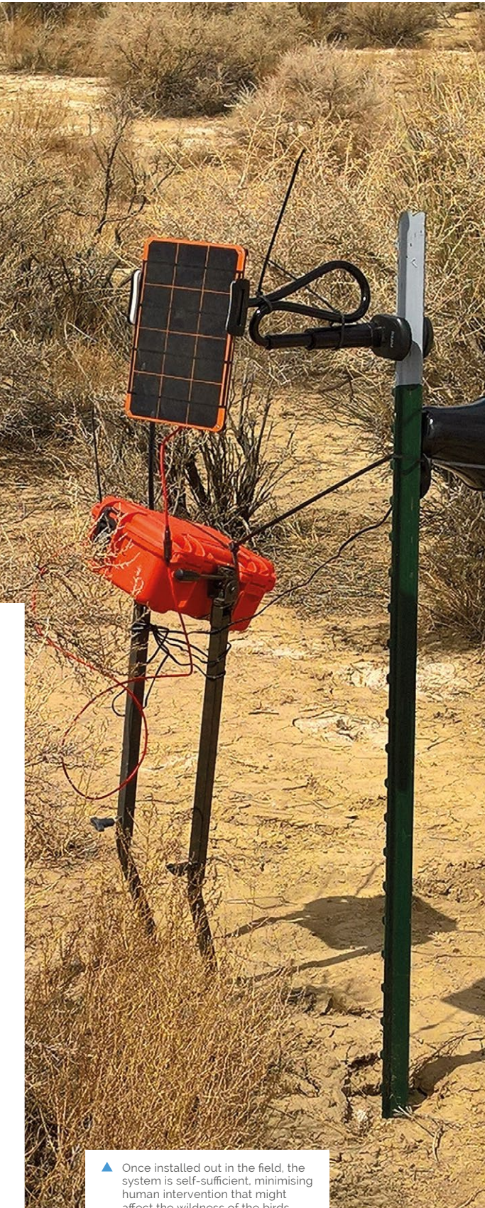
▲ A waterproof case keeps the electronic components safe in any weather conditions
