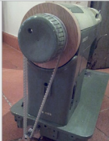
Above A modified handwheel is driven by a belt connected via a pulley system to a Nema 17 stepper motor, controlled using the z-axis in Grbl on the Arduino
