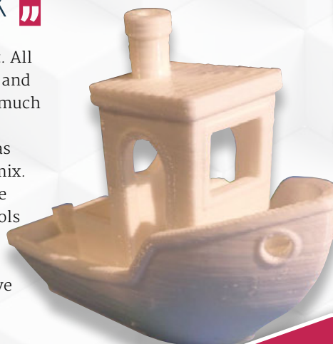
Above The 'Benchy' boat and Cali Cat are stress tests for your printer to check calibration, adhesion and temperature. You get some cute prints as a reward
