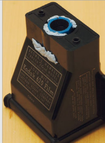
Above The webcam is inserted into the Kodak Brownie casing, but the camera's aperture doesn't allow light to fully expose the CCD chip, resulting in circular rather than rectangular images
