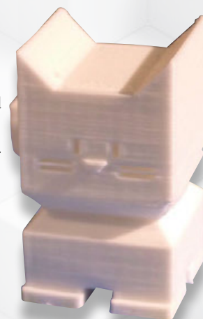
Above The 'Benchy' boat and Cali Cat are stress tests for your printer to check calibration, adhesion and temperature. You get some cute prints as a reward
