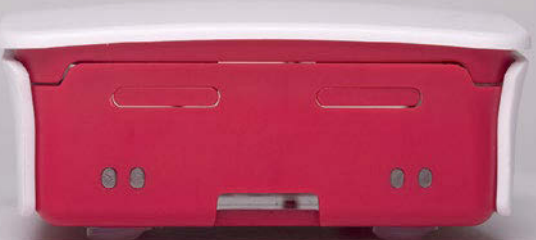
Above This fake case has two sets of light pipes Below The shoddy feet on this case are a clear sign of a fake
