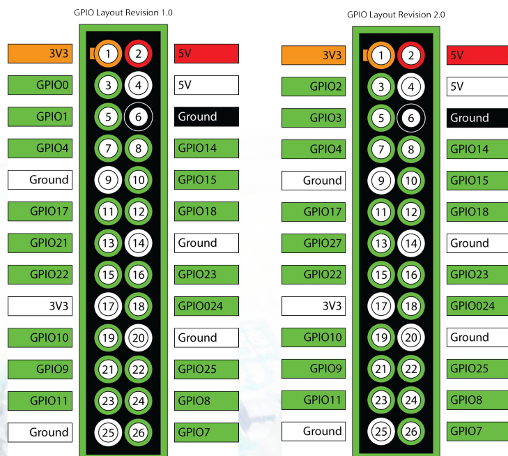
Please note GPIO reference changes for pins 3,5,7 & 13 on Revision 2.0
