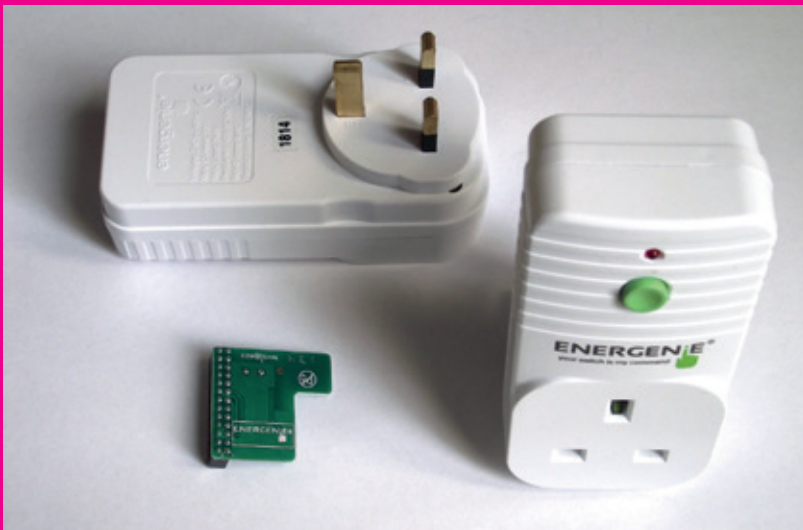
These Energenie sockets are two of the many types of you can control from OpenHAB.
