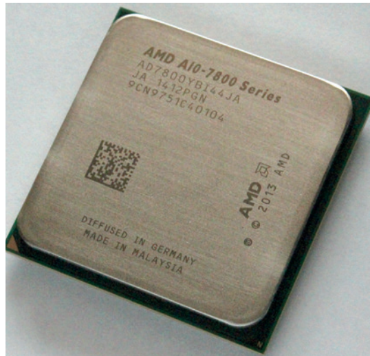
Most modern CPUs are in fact multiprocessors. This AMD A10 (Kaveri) chip is no exception: it has four CPU and eight GPU cores. Photo: Yulia Sinitsyna
